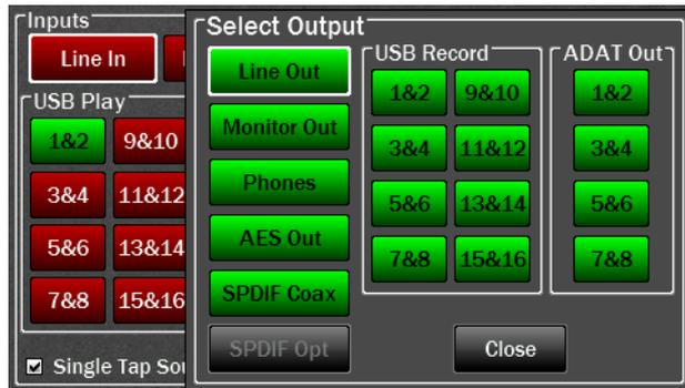
When the 16-channel USB Mode is engaged, all 16 USB input and output channels are visible and available.
