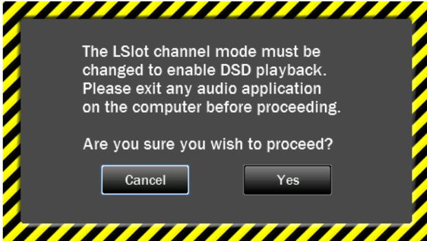
When switching into DSD Mode to “Auto”, if Hilo is in 16-channel LT-USB mode, then a warning screen will appear. As DSD requires a sample rate of 176.4kHz available only in USB 8-channel mode, this screen will prompt you to switch to 8-channel LT-USB mode.
