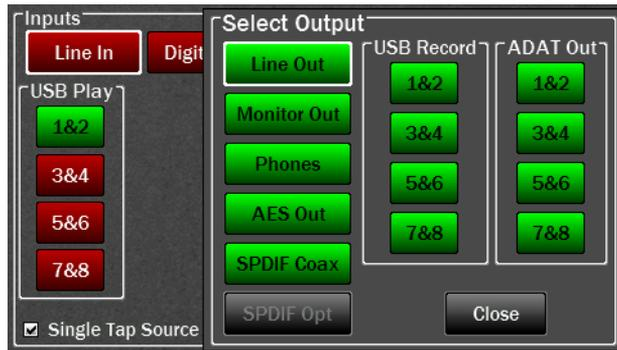
When Hilo is in 8-channel LT-USB Mode, USB channels 1-8 are visible and available.
