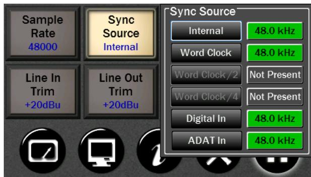
When the LT-USB is **NOT** connected to the computer, the Sync Source may be changed to one of the following four choices:
