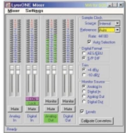
The Lynx One Mixer provides a comprehensive selection of options, along with 'zero'-latency monitoring facilities. Here you can see the useful indicators for the digital input in operation, showing that it is currently locked and receiving valid consumer audio data.
