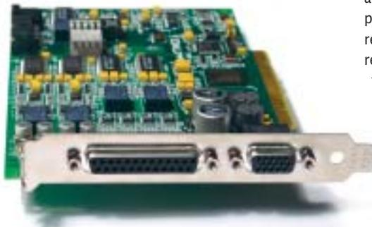
The Lynx Two's audio I/O reaches the card through breakout cables attached to these two D-type ports.
