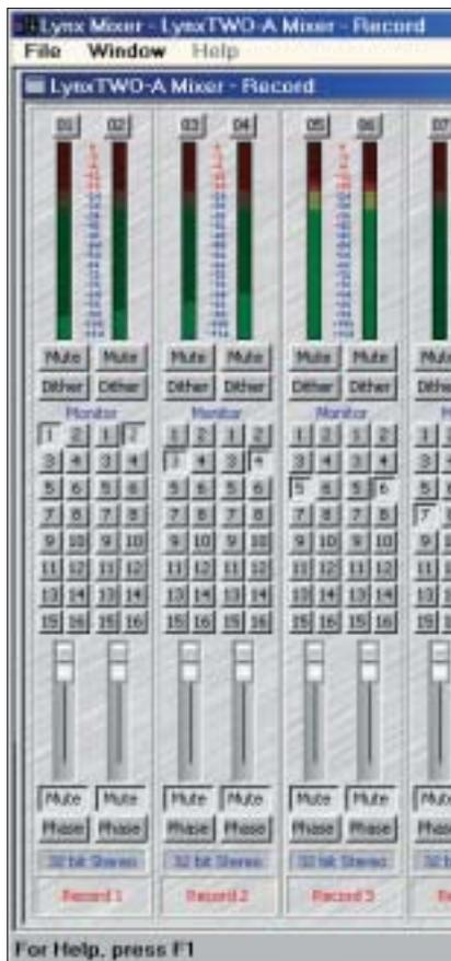
The Record Mixer window lets you select suitable input signals for each recording channel, as well as set up a complex monitoring mix to any combination of its various output sockets.
